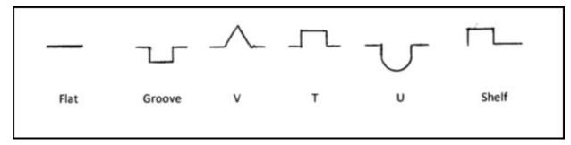
FIGURE 9: STANDARD BEVEL PROFILES
